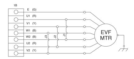
TB = TERMINAL BLOCK EVF MTR = EVAPORATOR FAN MOTOR
