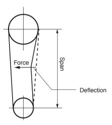
To measure belt tension, use a belt tensioner as shown in Figure 3. Determine actual deflection by depressing one belt with the belt tensioner and then adjust the belt tension to the correct pounds force and tighten all setscrews to the proper torques.
